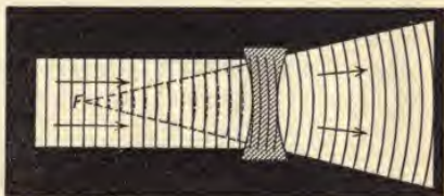
FIG. 238. — Parallel Rays of Light are Scattered by Concave Lenses.
